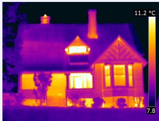
FIGURE 2: THERMAL IMAGE SHOWING AREAS OF ENERGY LEAKAGE AND HEAT LOSS (AREAS IN YELLOW ARE WARMER THAN THE AREAS IN PURPLE)
