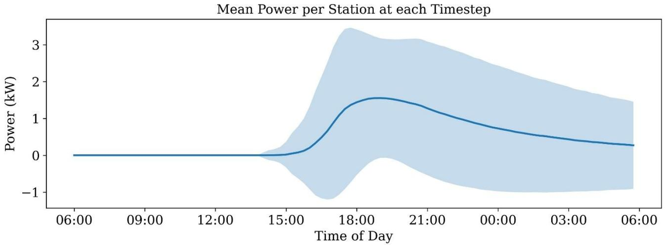
Figure 6: Mean power per circuit at each timestep in the simulation, with +/- 1 standard deviation shown in shading, for an example simulation of 4-way sharing on a 40A circuit for 40 VKT.
