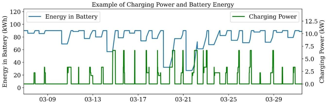
Figure 11: Charging power and energy in the battery of an example vehicle for a few simulated weeks in March 2019.
