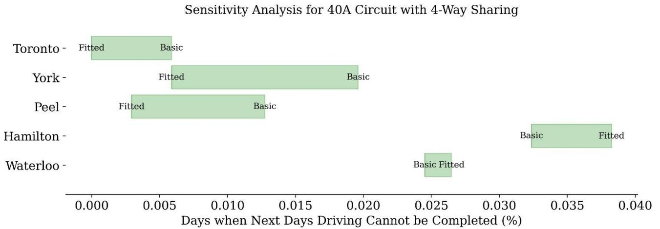
Figure 24: Sensitivity analysis of days when next day's driving cannot be completed for 40A circuit with 4-way sharing.
