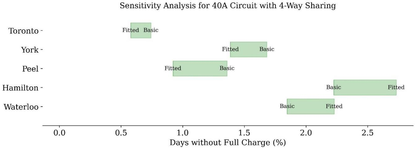
Figure 23: Sensitivity analysis of days when battery is not fully charged for 40A circuit with 4-way sharing.
