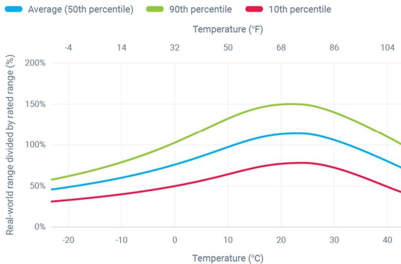
Figure 5: Real-world range compared to rated range of EVs. Reproduced from [7].
