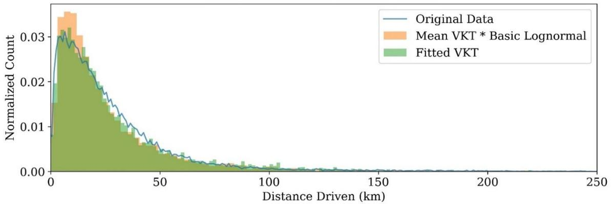
Figure 2: Example of the modelled distribution (orange) compared to the actual data (blue) and a fitted lognormal distribution (green) for Toronto.
