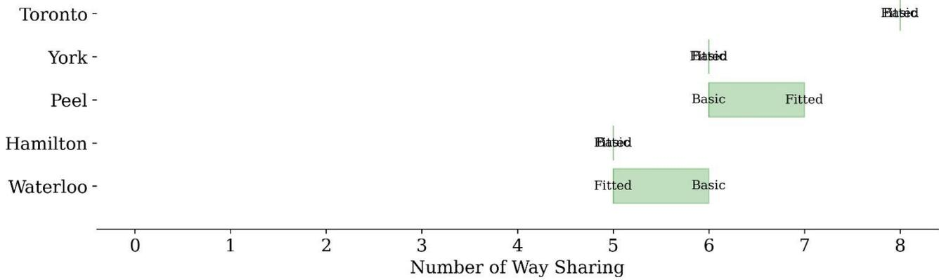
Figure 25: Sensitivity analysis of maximum sharing on a 40A circuit with specified metric thresholds.
