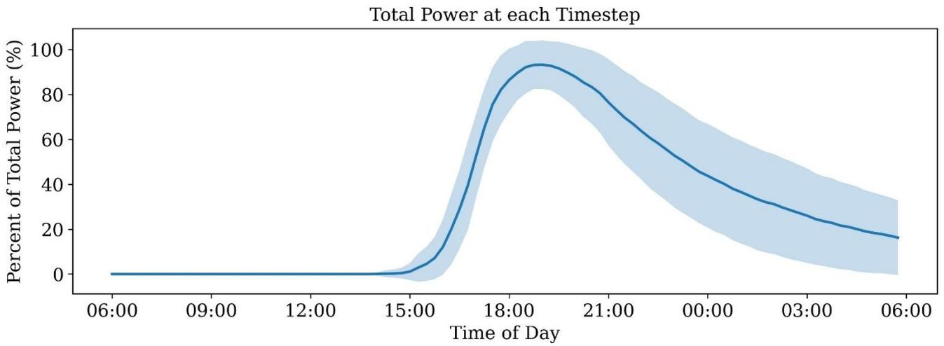
Figure 7: Mean percent of total available power used at each timestep in the simulation, with +/- 1 standard deviation shown in shading, for an example simulation of 4-way sharing on a 40A circuit for 40 VKT.
