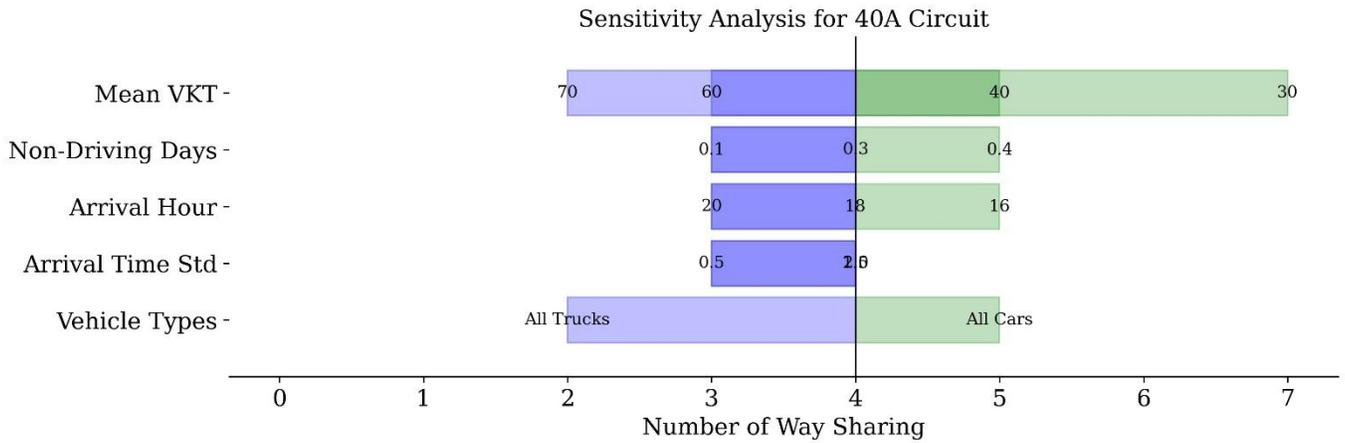
Figure 14: Sensitivity analysis of maximum sharing on a 40A circuit with specified metric thresholds.
