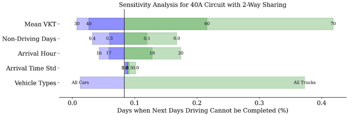
Figure 13: Sensitivity analysis of days when next day's driving cannot be completed for 40A circuit with 2-way sharing.
