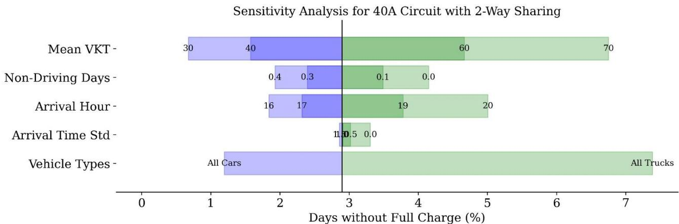
Figure 12: Sensitivity analysis of days without full charge for 40A circuit with 2-way sharing.
