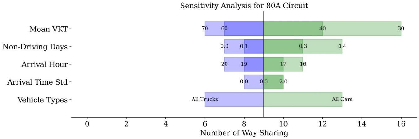
Figure 15: Sensitivity analysis of maximum sharing on an 80A circuit with specified metric thresholds.
