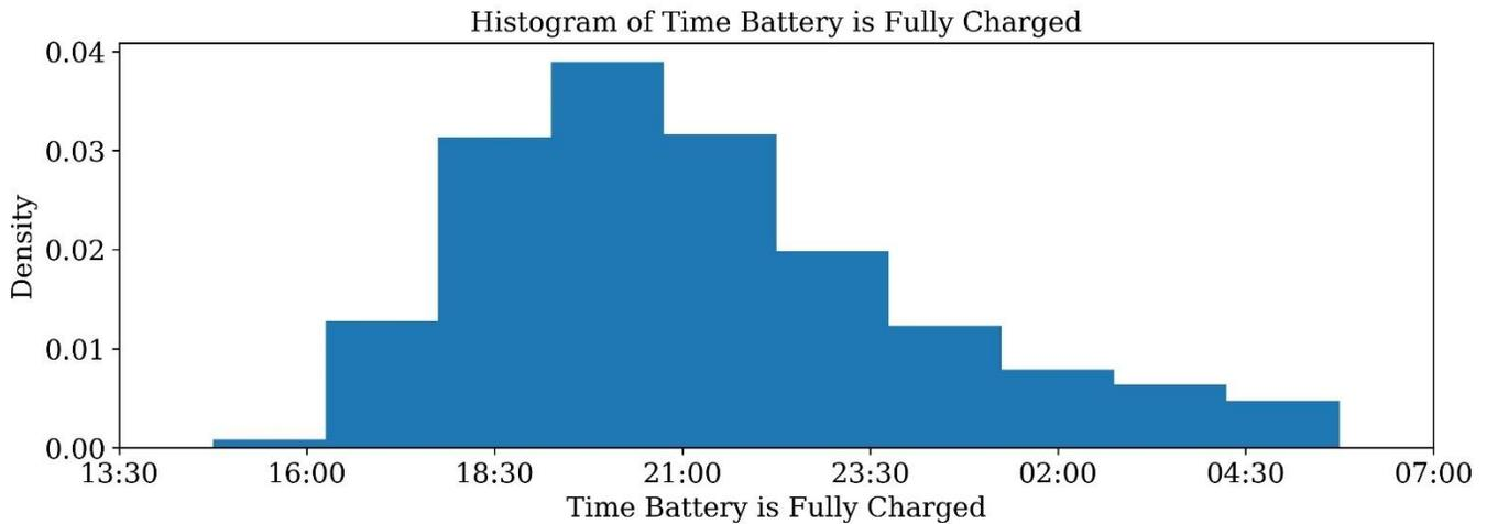
Figure 8: Histogram of time that batteries are fully charged for an example simulation of 4-way sharing on a 40A circuit for 40 VKT.
